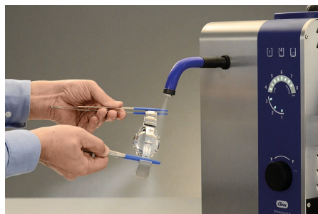
Cleaning with flexible handpiece Parts can be held securely (also with tweezers) and sprayed all-round quickly and effectively.
